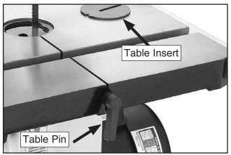
Figure 50. Table insert and table pin.
